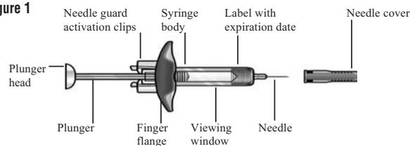
**Do not touch the needle guard activation clips** to prevent premature activation of the needle safety guard.
